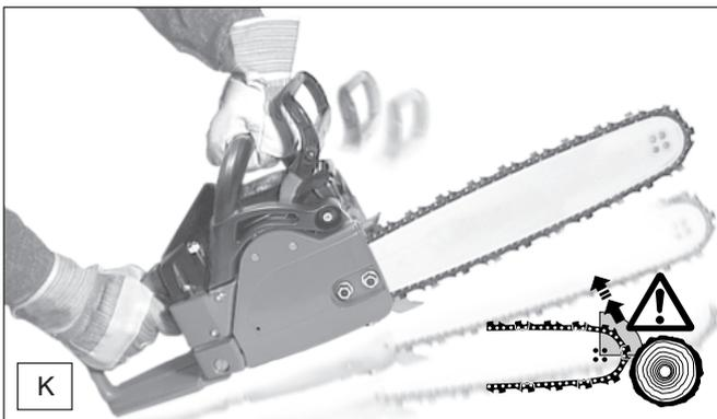
The MAKITA models comes with an inertia chain brake as standard equipment. If kickback occurs due to contact of the guide-bar tip with wood (see SAFETY PRECAUTIONS), the chain brake will stop the chain through inertia if the kickback is sufficiently strong. The chain will stop within a fraction of a second.
