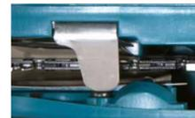
Tool-less saw chain tension adjustment
